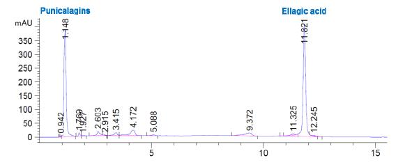
**Figure 1**. HPLC profile of pomegranate juice at 254 nm. Punicalagins (1.148 min) and ellagin acid (11.821 min) were identified comparing retention times and UV-visible spectra with standards analysed by the same method.
