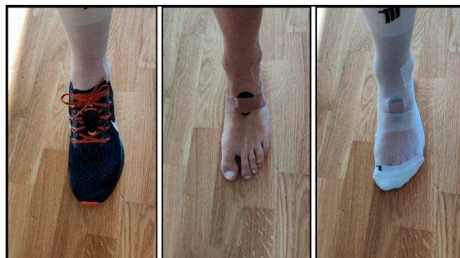
Figure 1. Representation for the placement of the Stryd™ power meter clipped on the laces of the runner's shoe (left picture) and placed and secured with tape on the runner's instep during barefoot running (central and right picture).
