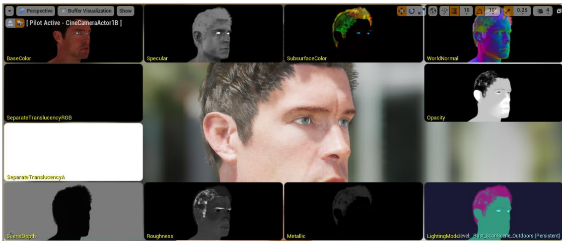
Figure 4: GBuffer combination to produce a high-quality Render image in Unreal Engine 4 Deferred Rendering System.
