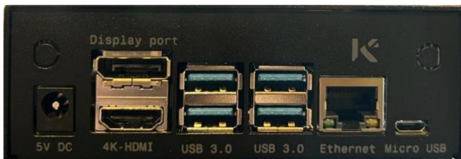
Figura 22: Puertos de NVIDIA Jetson Nano
